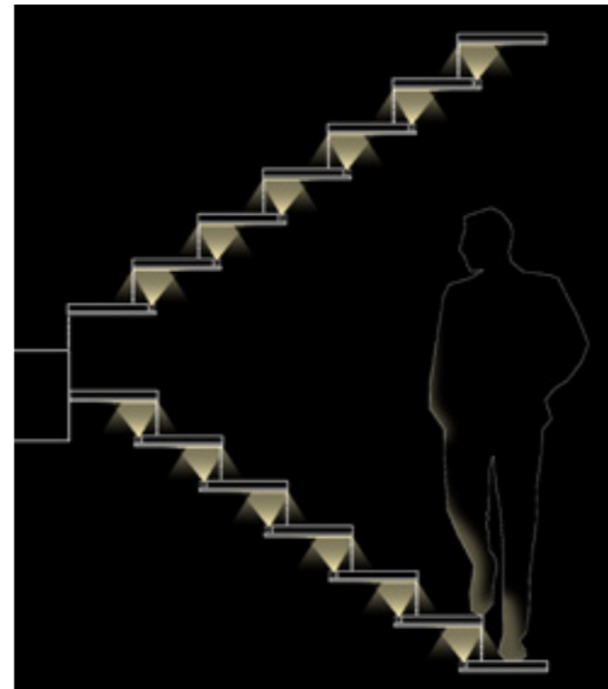
Diagram indicating feature core stair lighting principle
