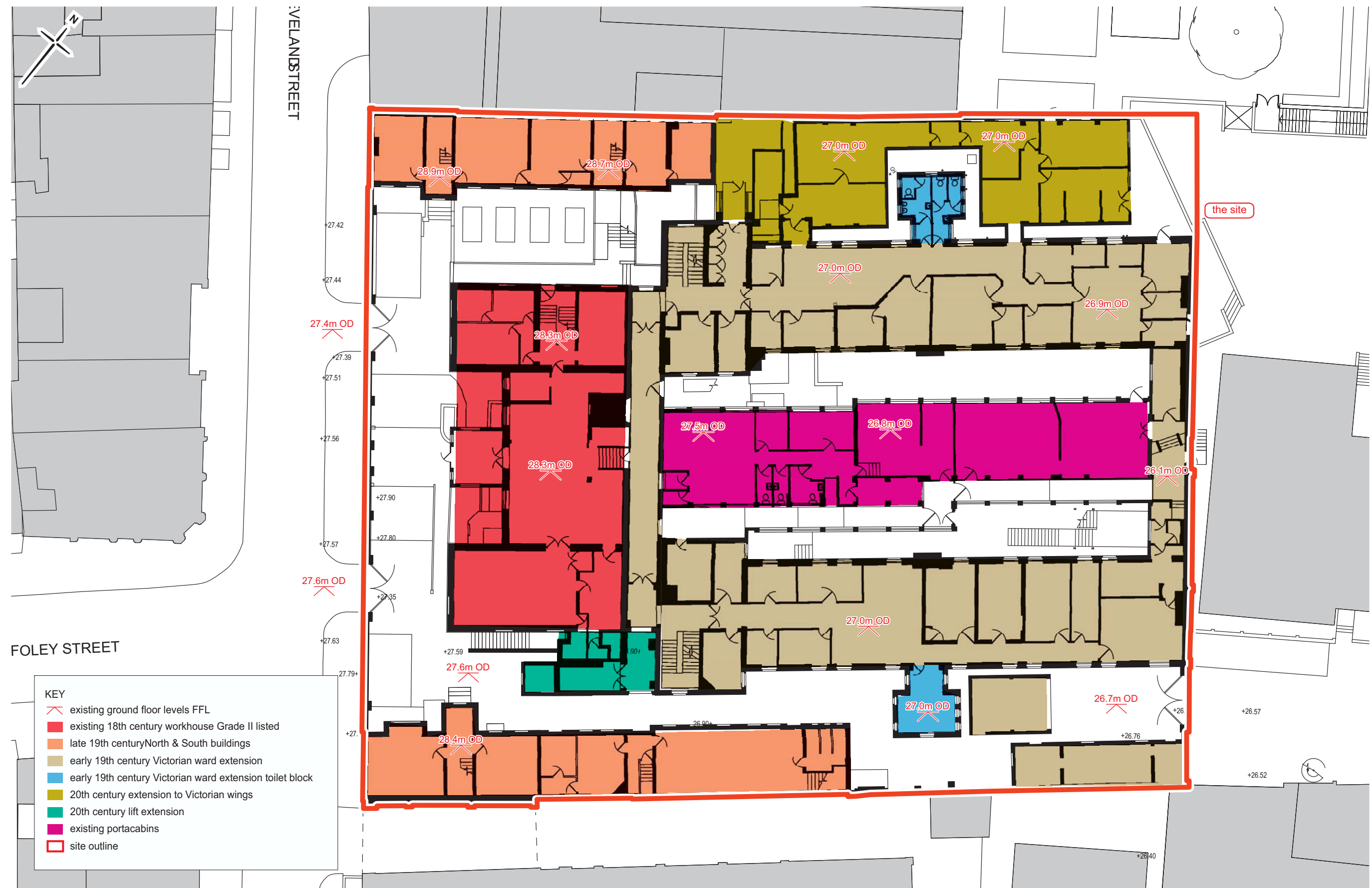
Fig 13 Existing ground floor plan, showing extent of current buildings on the site (Llewelyn Davies, LD15 078.00, drwg no P-XTG-L00 dated 20-1-2017), with known ground levels taken from Topographical Survey (Greenhatch group, drwg no 13514_09_P, rev C, 10-06-2017)
