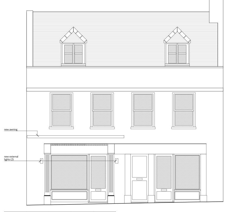
Full cassette traditional awning with white powder coated aluminum frame and cassette. Fabric in Teflon coated awning canvas, light grey. Awning screwed to the brickwork above the fascia with nylon rawl plugs.
