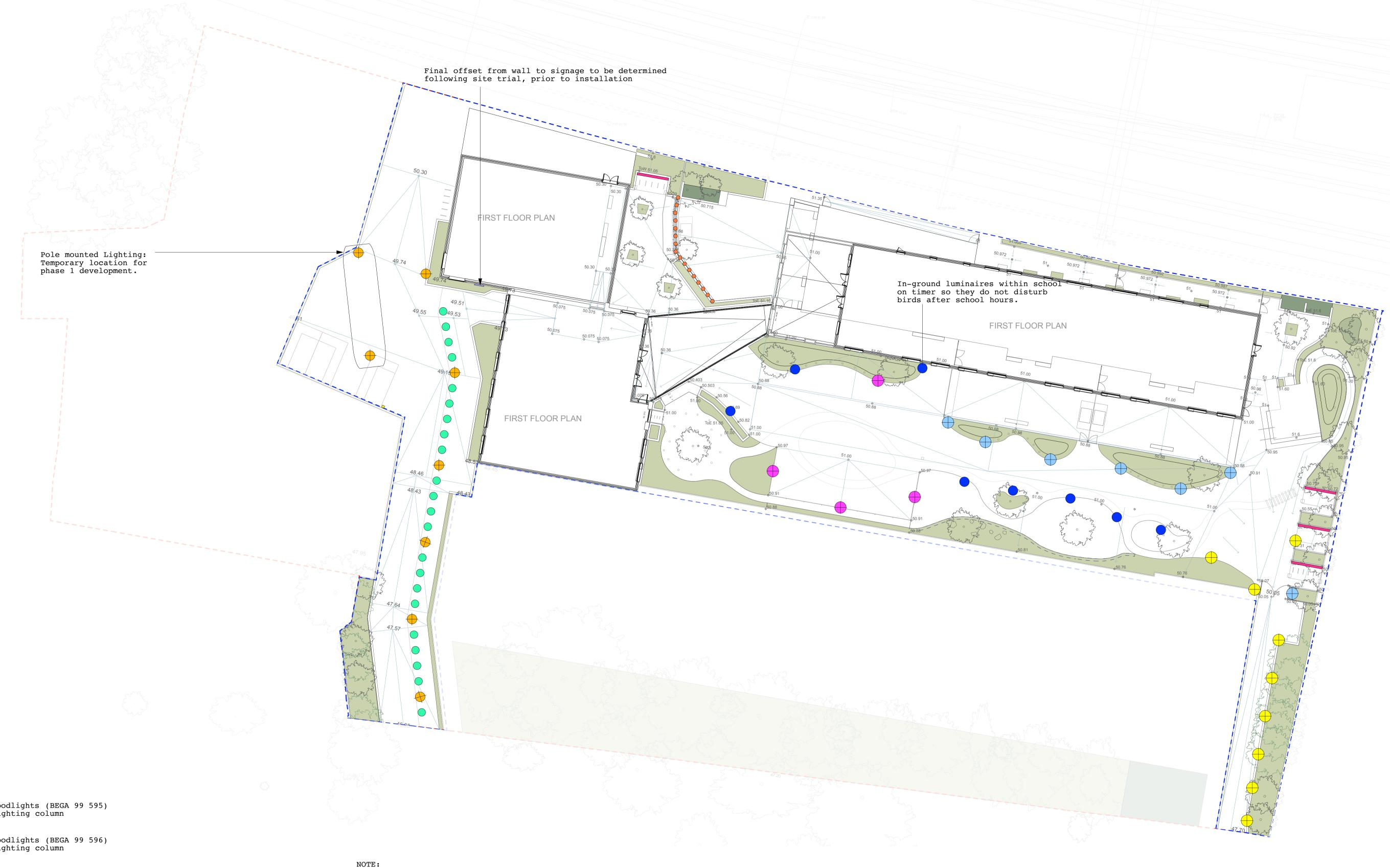
Pole mounted floodlights (BEGA 99 595) mounted to 6m lighting column
