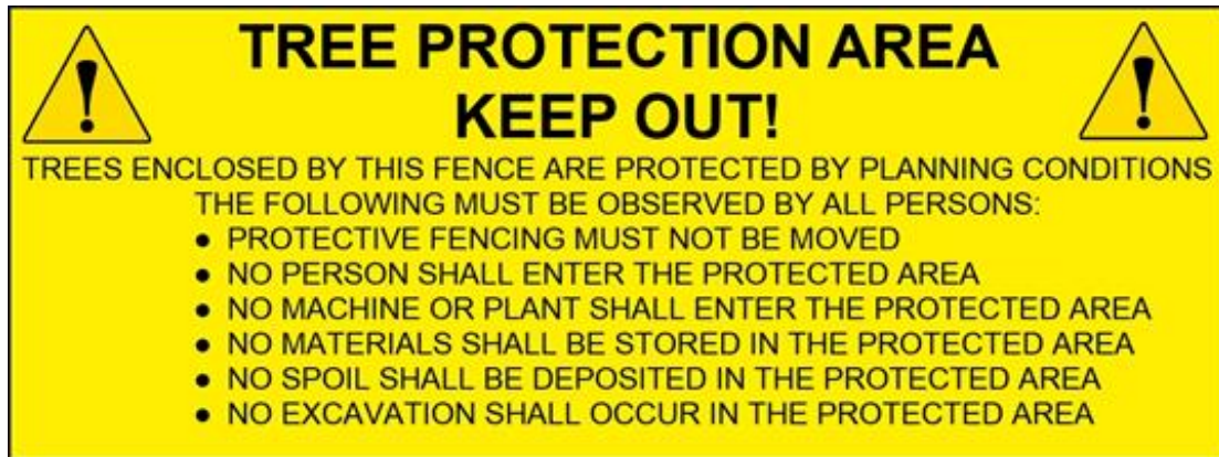
Figure 2. Wording to be included in high visibility all-weather sign attached to protective fencing
