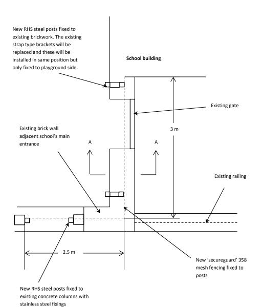
New 'secureguard' 358 mesh fencing fixed to posts **New RHS steel posts** fixed onto existing brick wall 3.6 m School's playground Existing brick wall adjacent school's main entrance
