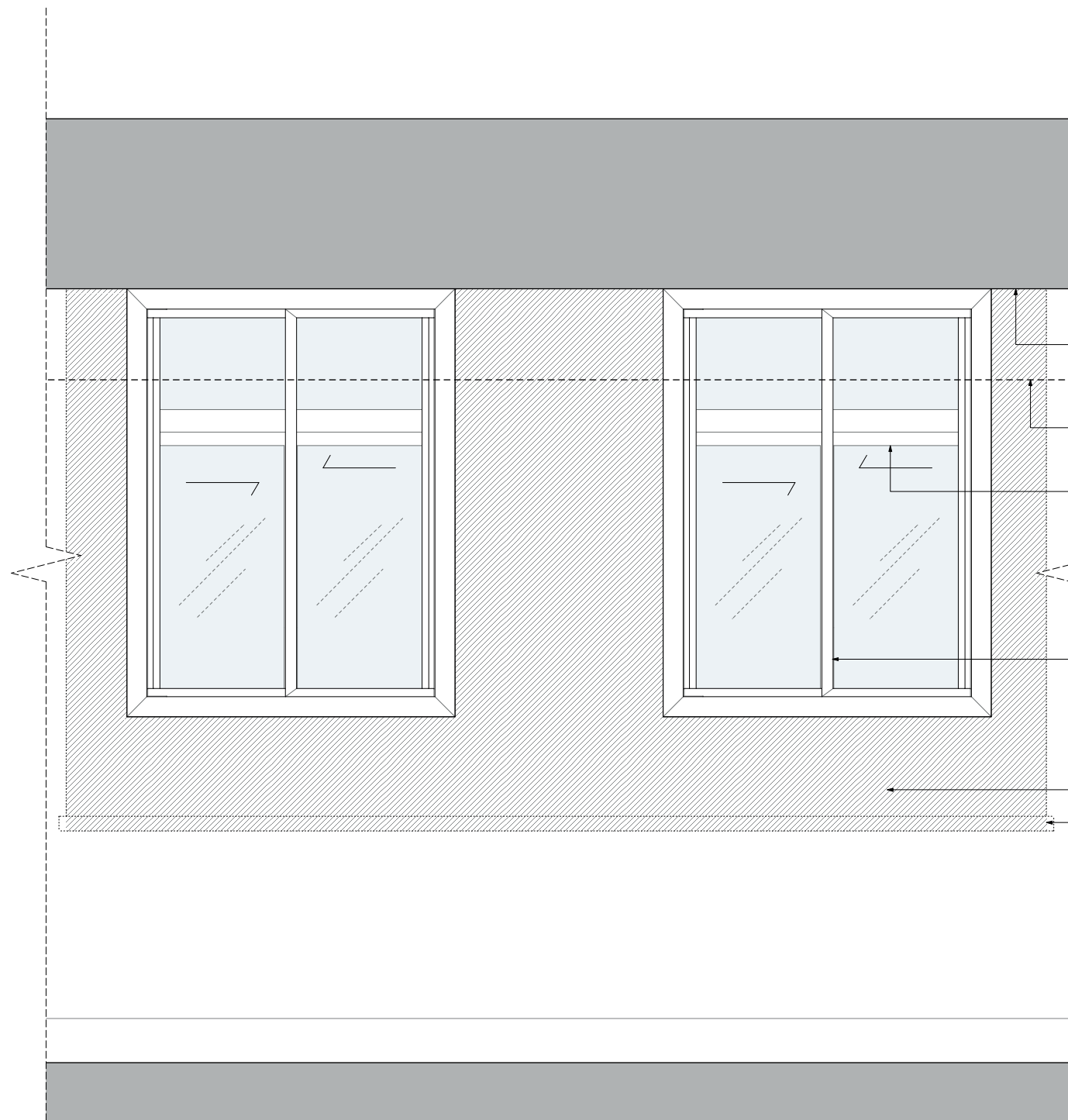
2 Secondary Glazing Type C: Proposed Internal Elevation 1:10 at A1
