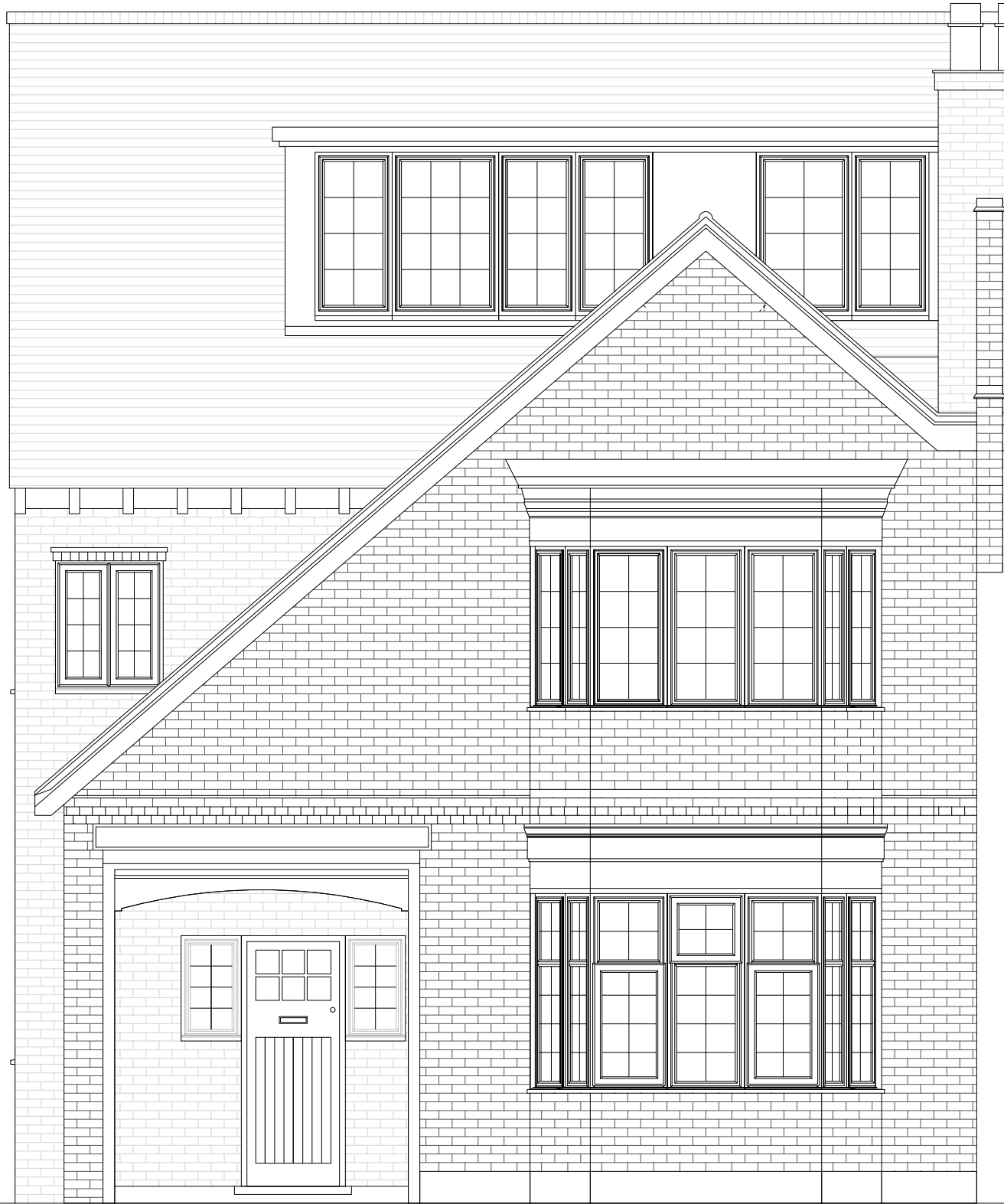
01 EXISTING : FRONT ELEVATION 1:50
