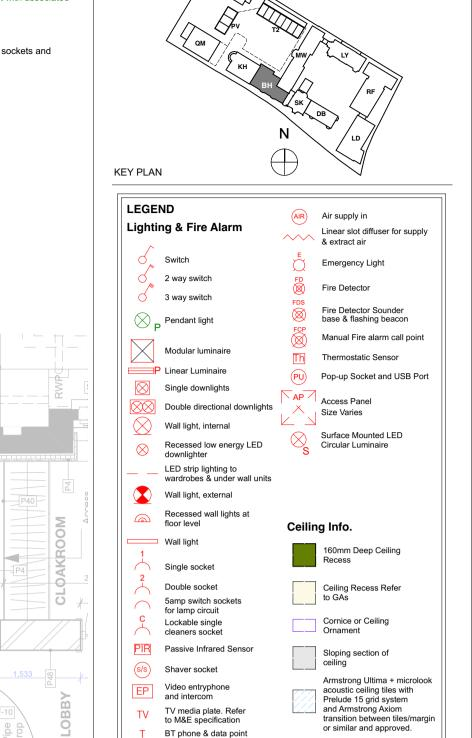
TV media plate. Refer to M&E specification BT phone & data point Floor recessed outlet
