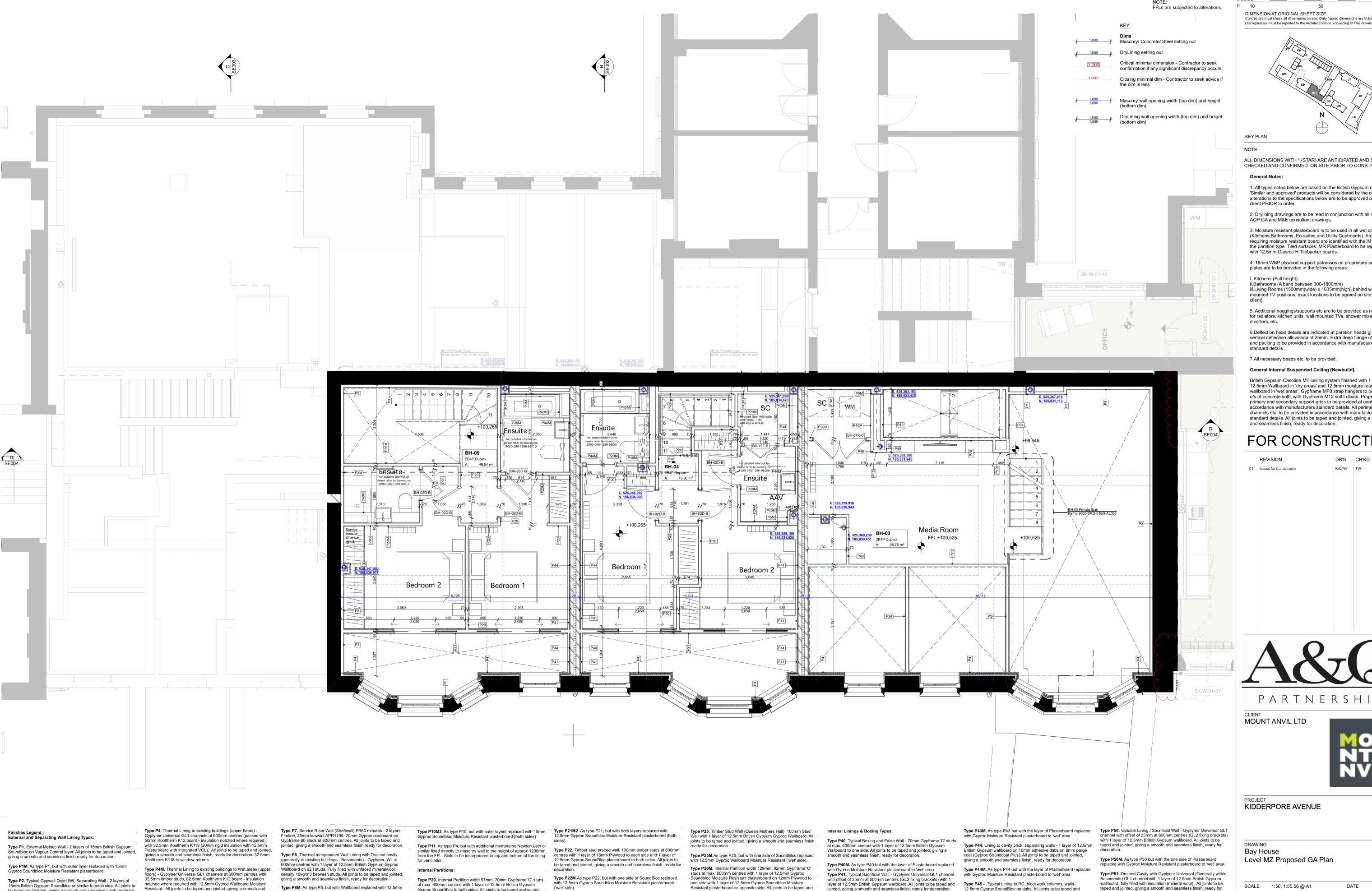
15mm British Gypsum Soundbloc or similar to each side. All joints to be taped and jointed, giving a smooth and seamless finish ready for
