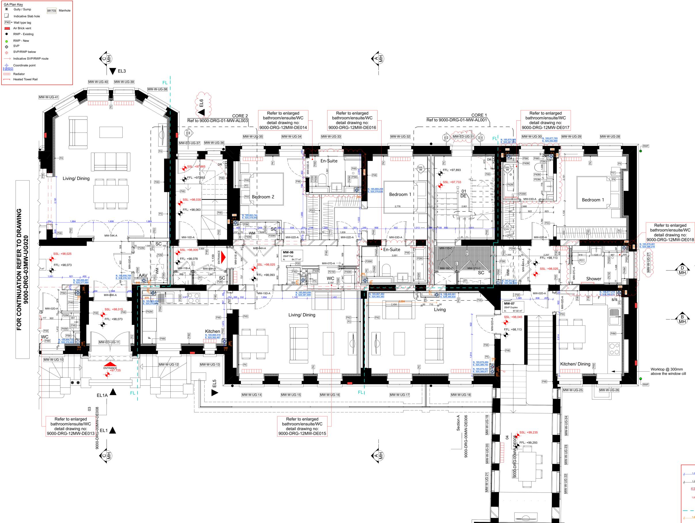
Finishes Legend : External and Separating Wall Lining Types: Type P1. External Metsec Wall - 2 layers of 15mm British Gypsum Soundbloc on Vapour Control layer. All joints to be taped and jointed,
