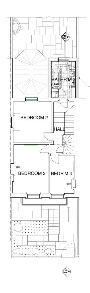
New Bathroom extension of cavity wall of fairfaced reclamed brickwork to match existing, blockwork and plaster internally.
