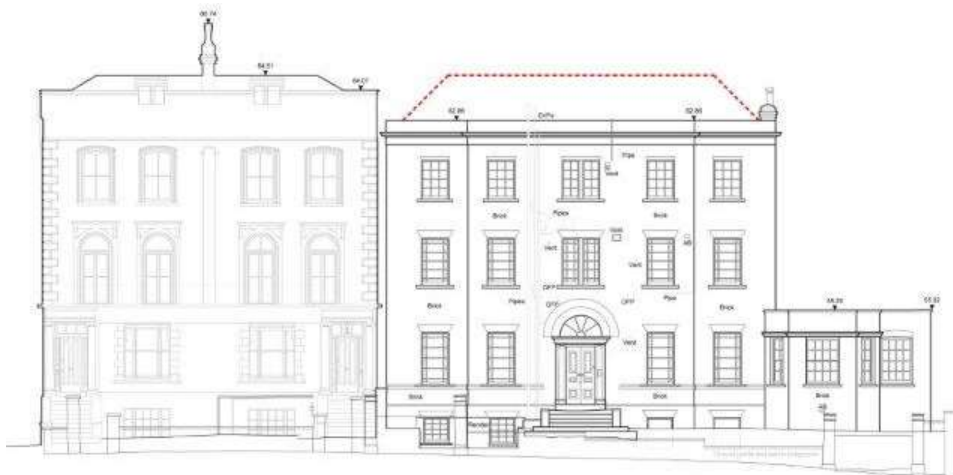
Fig 89: Elevation diagram showing potential for rebalancing the scale relationship with Lynton Villas
