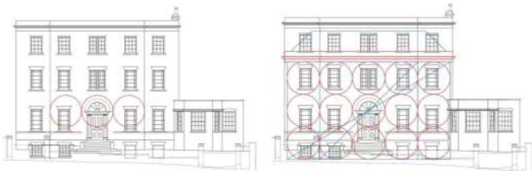
Fig 54 & 55: Proportion study. Right hand image shows original cornice line and roof profile
