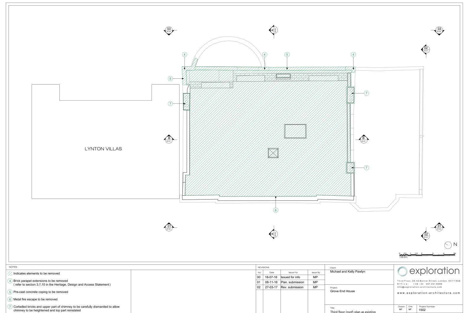
8 Felt roofing to be removed from parapet upstand and parapet top (refer to section 3.7.8 in the Heritage, Design and Access Statement)
