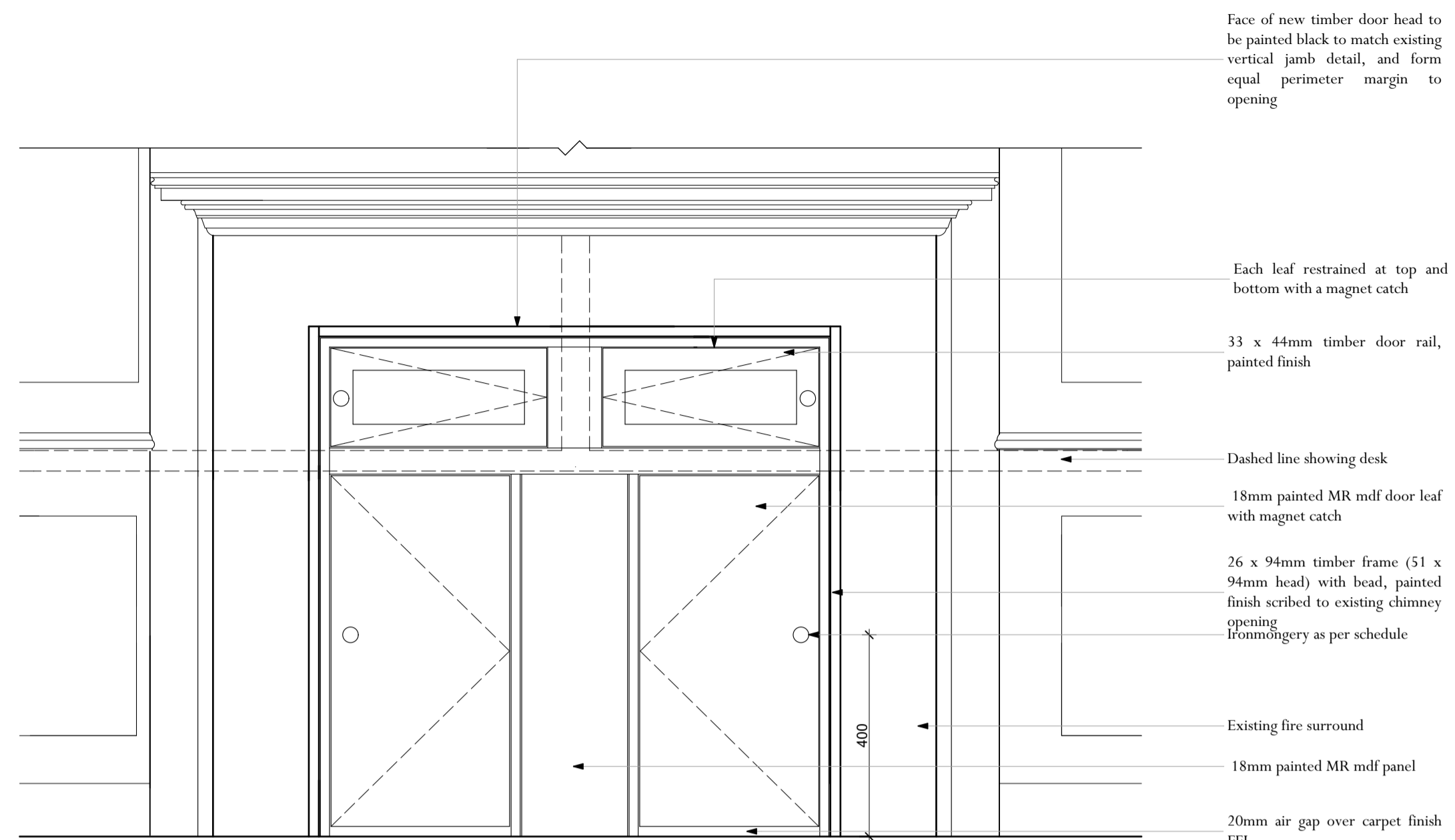
1:10 Studio Chimney Elevation
