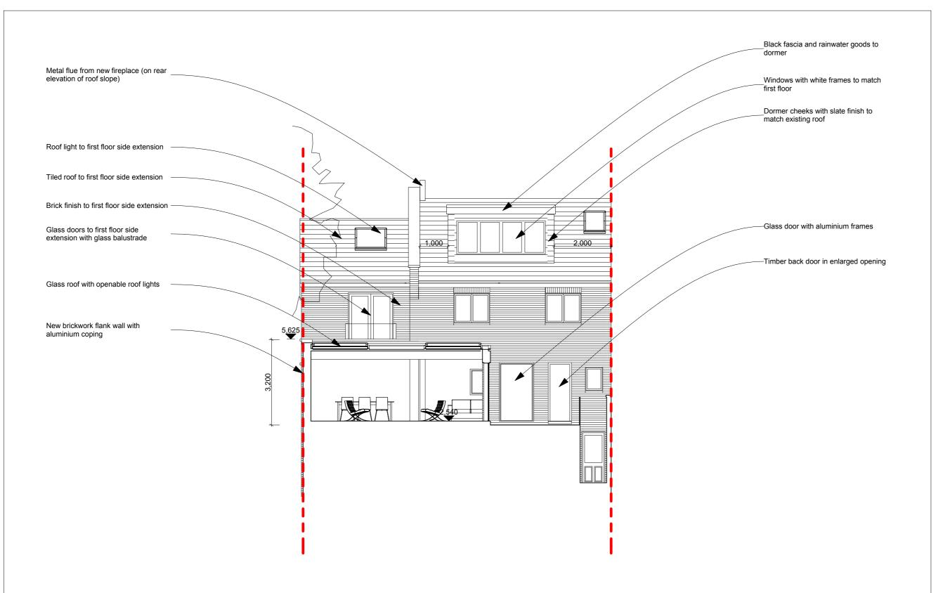
No implied licence exists. This drawing should not be used to calculate areas for the purposes of valuation. Do not scale this drawing. All dimensions to be checked on site by the contractor and such dimensions to be their responsibility. All work must comply with relevant British Standards and Building Regulations requirements. Drawing errors and omissions to be reported to the architect.
