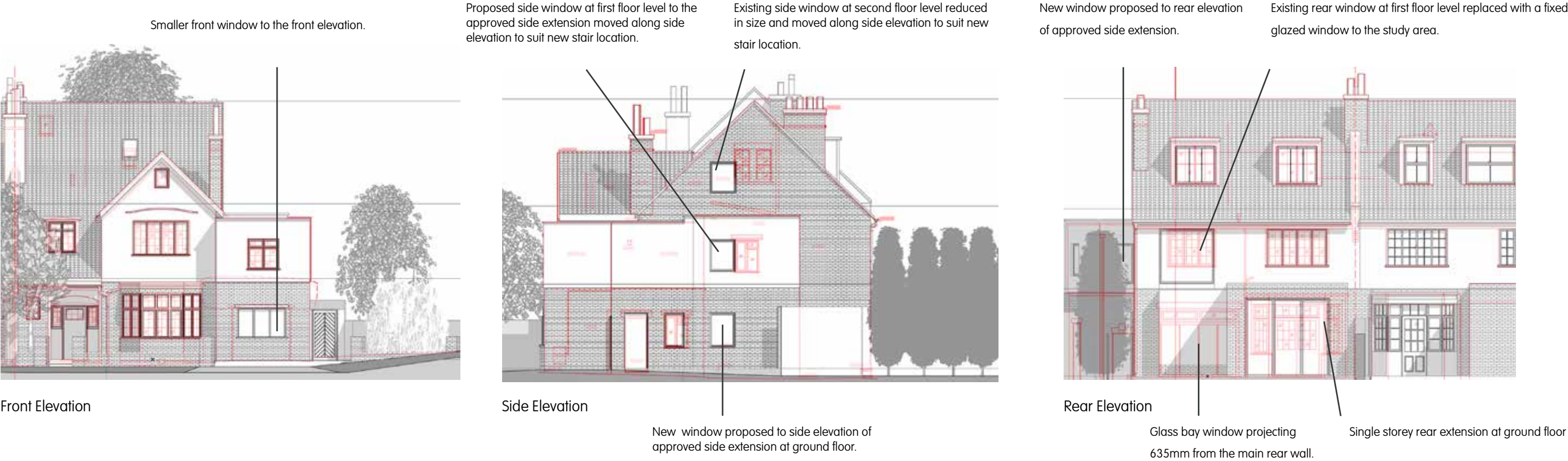
Figure 8: Proposed elevations showing the 2016/3129/P approved elevations overlay in red and identifying changes to previously approved side application.
