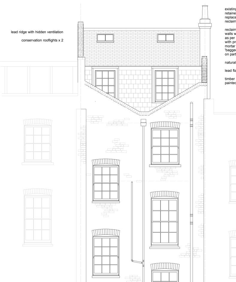
existing original chimney pots retained and reused, poor later replacement pots replaced with reclaimed pots to match originals
