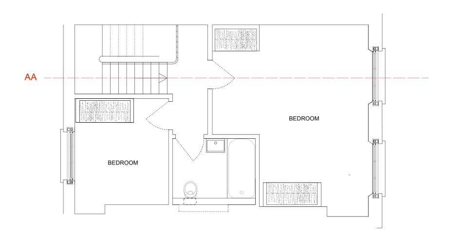
original existing stair new plasterwork reinstated throughout (2014) new bathroom enclosure modifies original planform original sash windows timber flooring throughout
