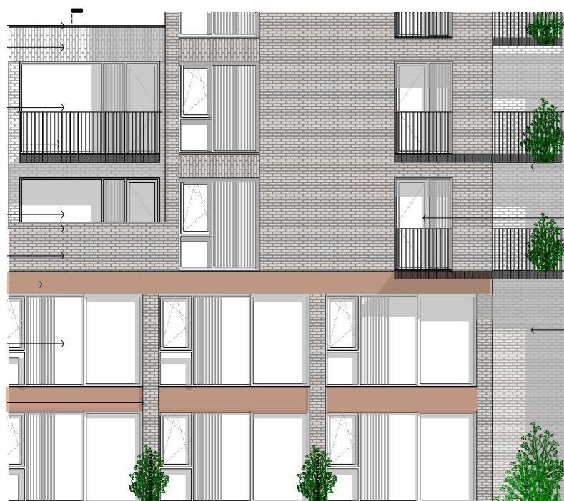
● Area of concrete proposed to be replaced with brick
