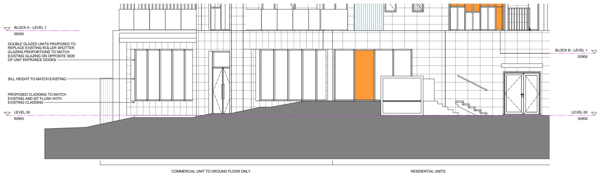
2 GA - EAST ELEVATION - COMMERCIAL UNIT - PROPOSED
