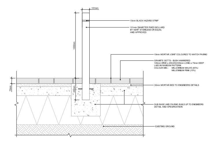
F04 SECTION THROUGH FIXED BOLLARD 1:15 @ A3
