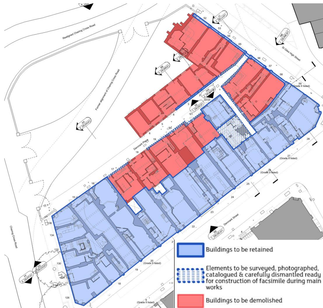
Figure 8.1: Extent of demolitions.
