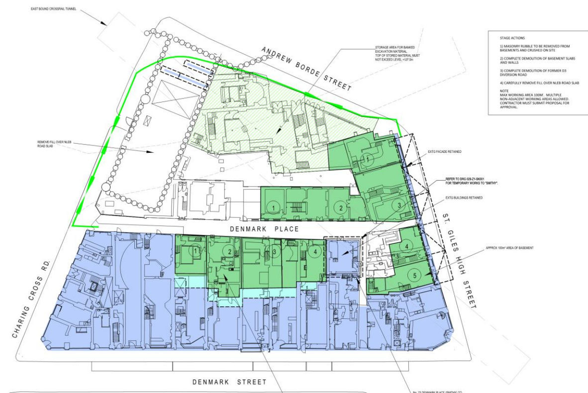
Figure 8.3: Breaking out of basements to be conducted in hit and miss arrangement.
