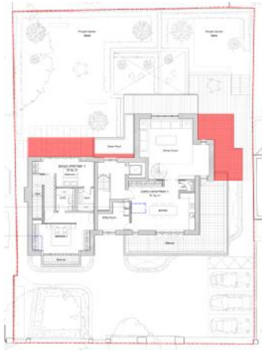
Image: floorplan showing the extent of cutbacks on the second floor level.
