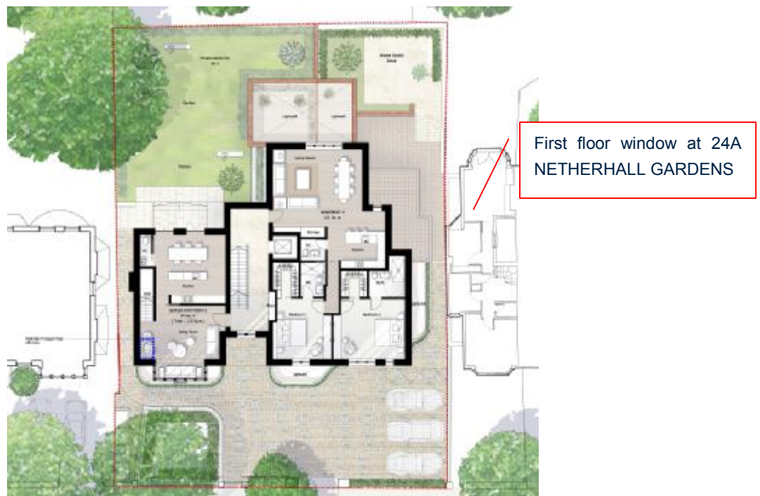
Image: first floor plan showing that a 45 degree angle view is achieved from the first floor window at 24a Netherhall Gardens.
