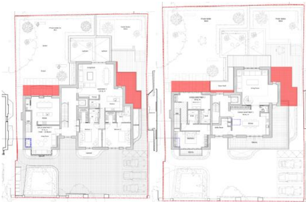
Images: floor plans showing the extent of cutbacks on the first and second floor levels.
