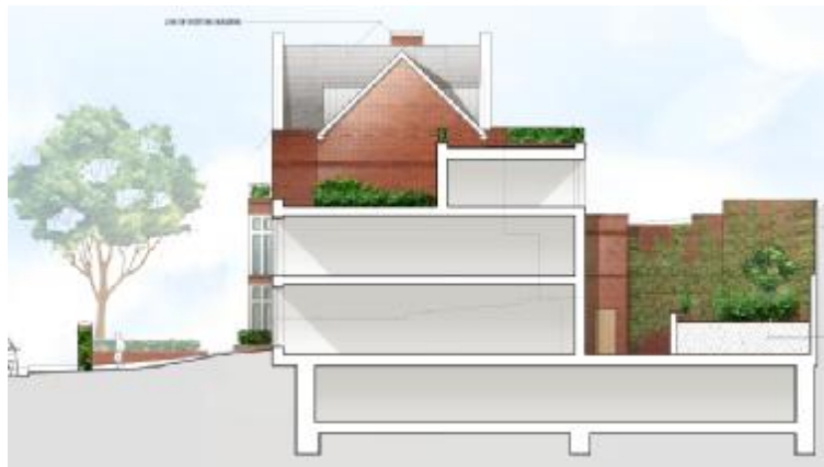
Image: section illustrating the lower ground, ground, first, second and third (within roof) floor levels.
