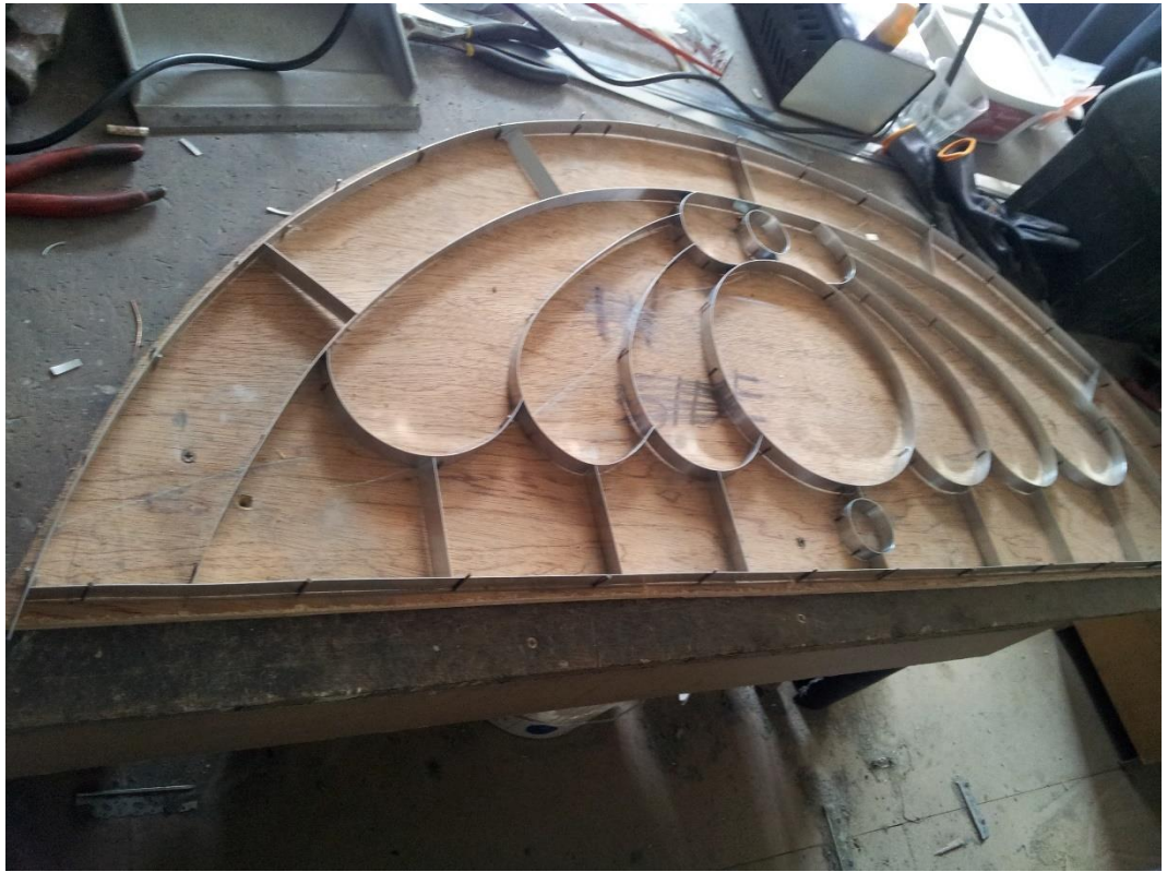
Zinc framework under assembly in workshop
