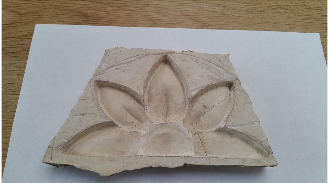
Typical plaster mould for lead casting. NB Leaf positions will differ.
