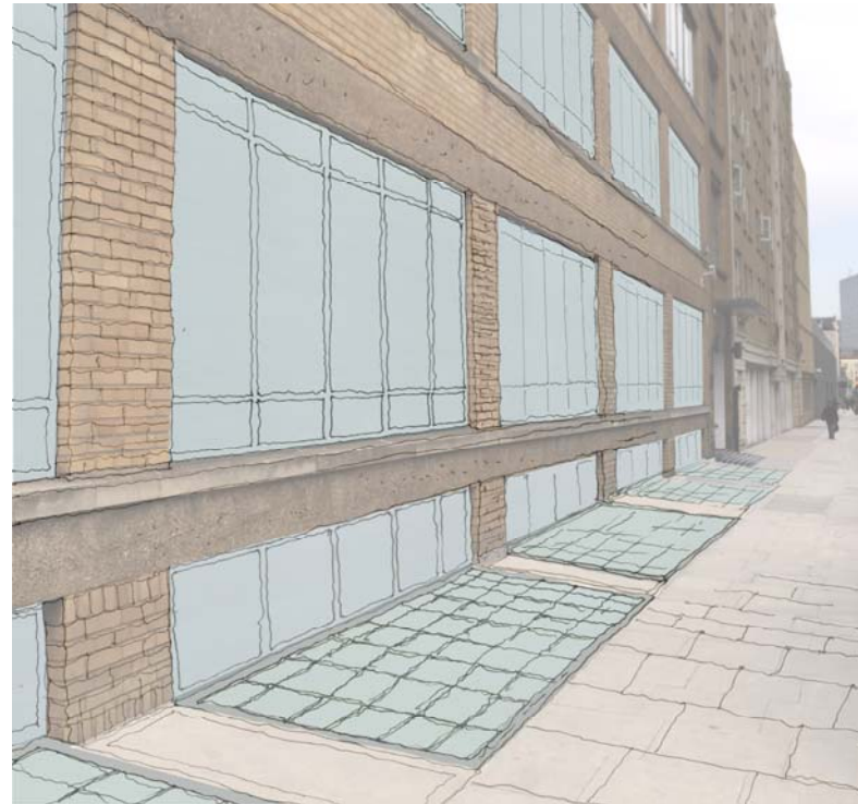
Sketch of new low level metal framed glazing and cast iron pavement lights
