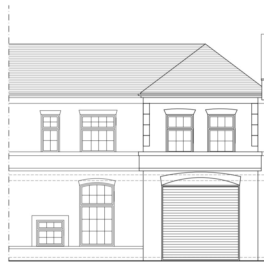
EXISTING FRONT ELEVATION
