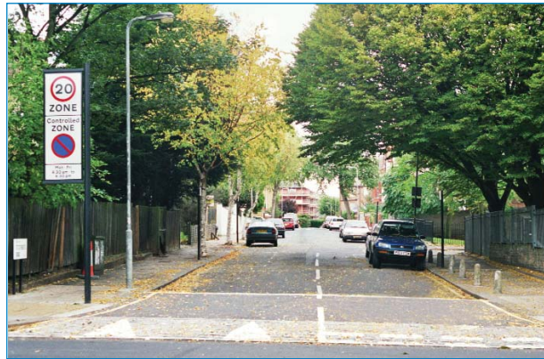
Raised entry treatment in St Cuthberts Road
