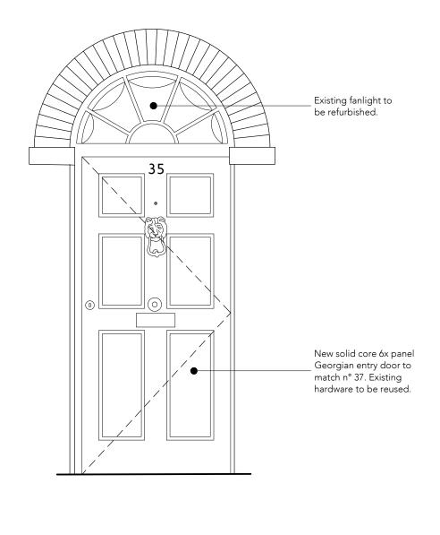
1 PROPOSED ENTRY DOOR DETAIL ELEVATION scale 1:20
