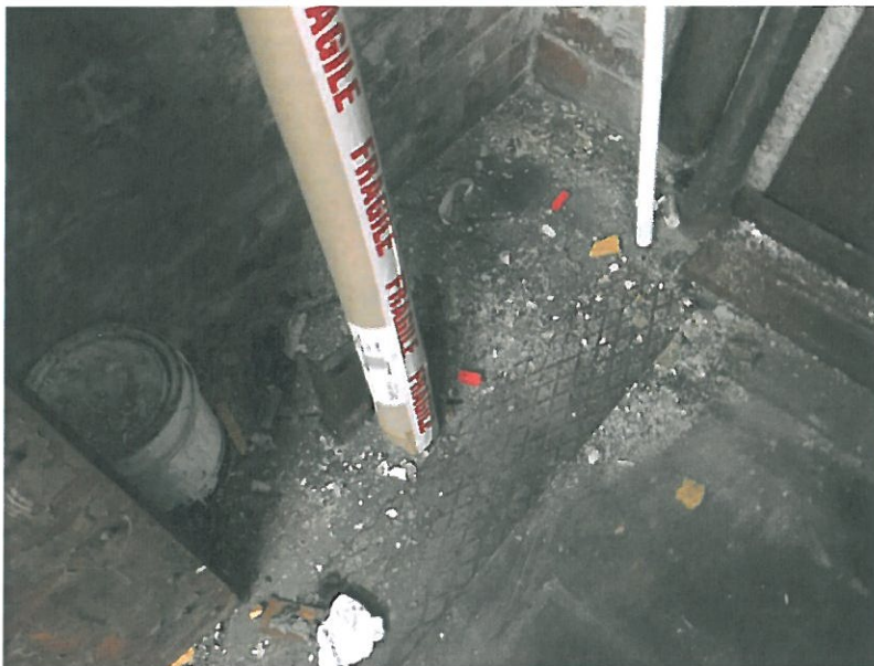
Sample 06 – Debris to floor – No asbestos detected.
