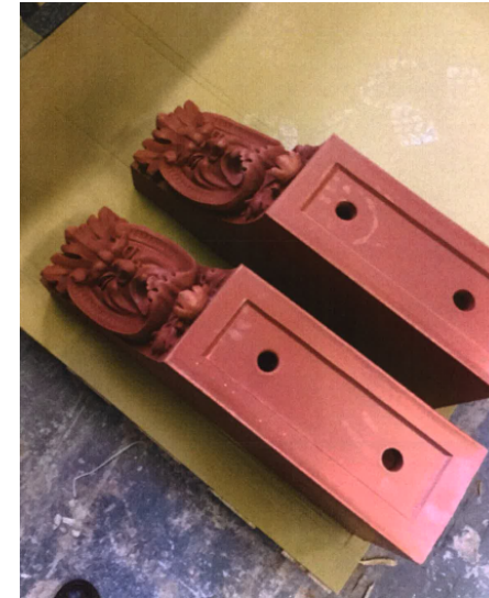
Terracotta Manufacture (Darwen) – Corbels to Bernard Street (2 nd Floor)
