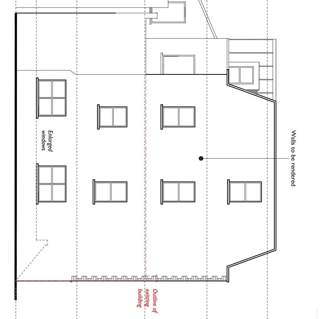
Proposed Rear Elevation - (North)
