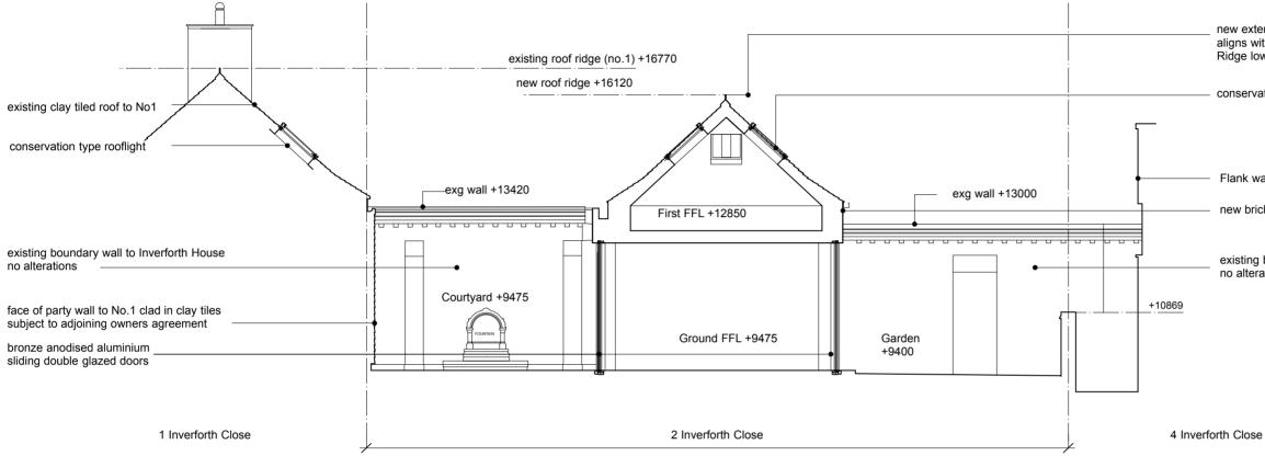
Proposed Courtyard North Elevation Scale: 1:100
