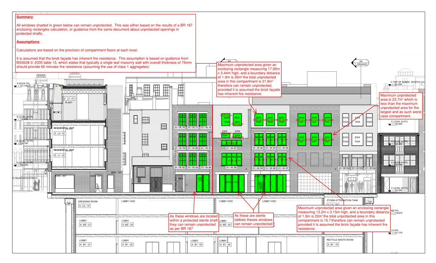
Figure 9—3 External Fire Spread – Block C North Elevation
