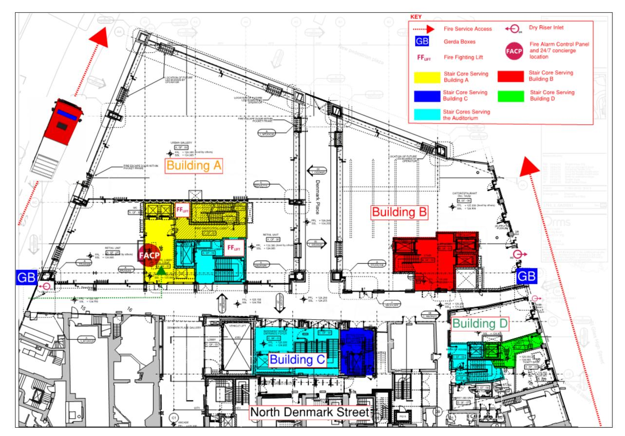
Figure 3—2: Locations for Dry Riser Inlets
