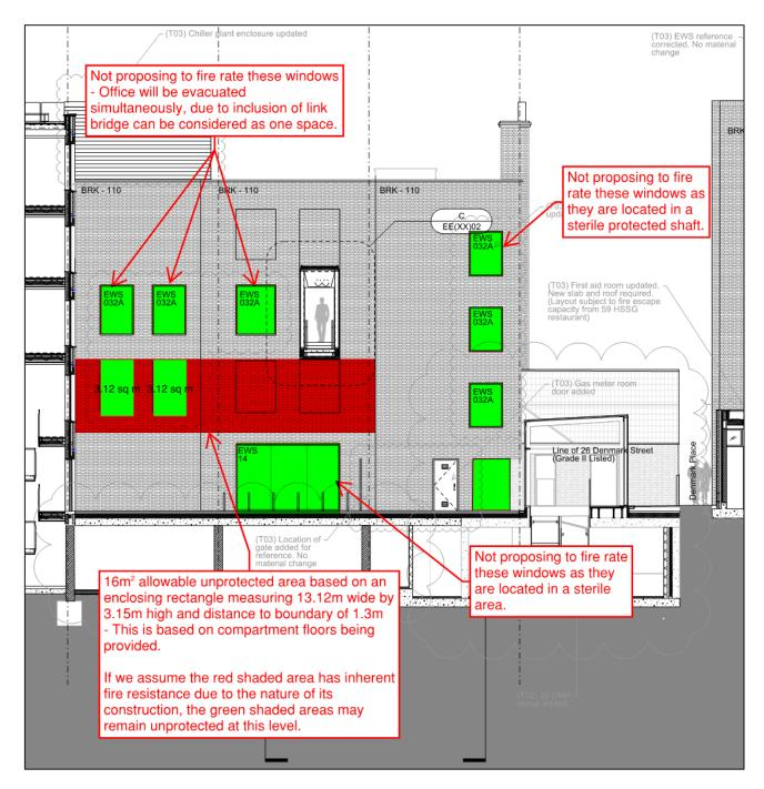
Figure 9—4 External Fire Spread – Block C South Elevation
