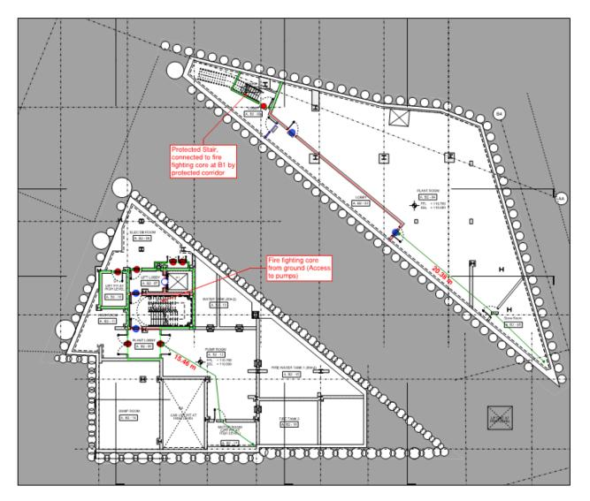
Figure 4-2: Level 2 Basement, showing protected stair and FF core
