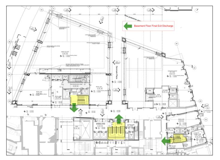
Figure 4—4: Ground Floor discharge points from basement stairs
