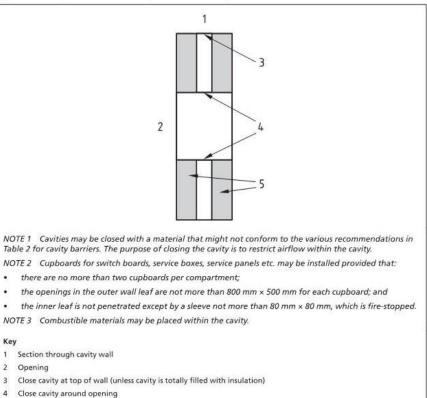
5 Two leaves of brick or concrete each at least 75 mm thick
