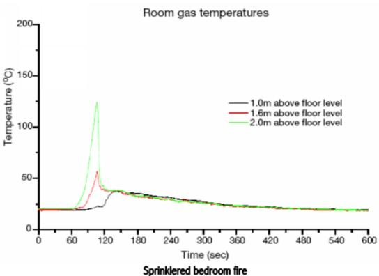
Room gas temperatures peaked at 125 deg C at 2m above floor level. At head height temperatures in the room
