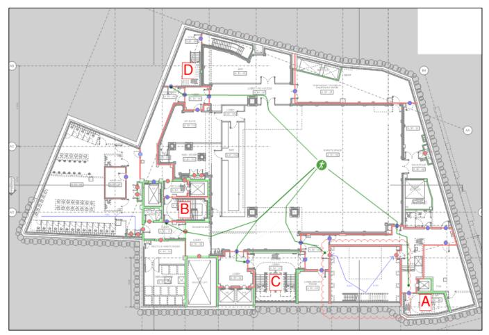
Figure 4—3: Level 1 Basement layout with egress routes and worst-case fire location
