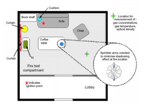
A concealed sprinkler was used in the tests. The results are summarised below:
