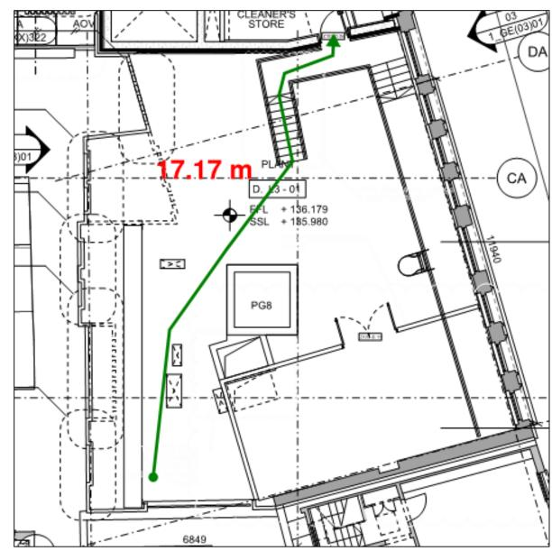
Figure 8—3: Level 3 plant room travel distance
