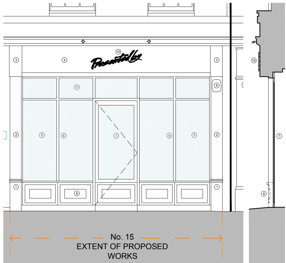
SHOPFRONT ELEVATION & SECTION @ 1:50
