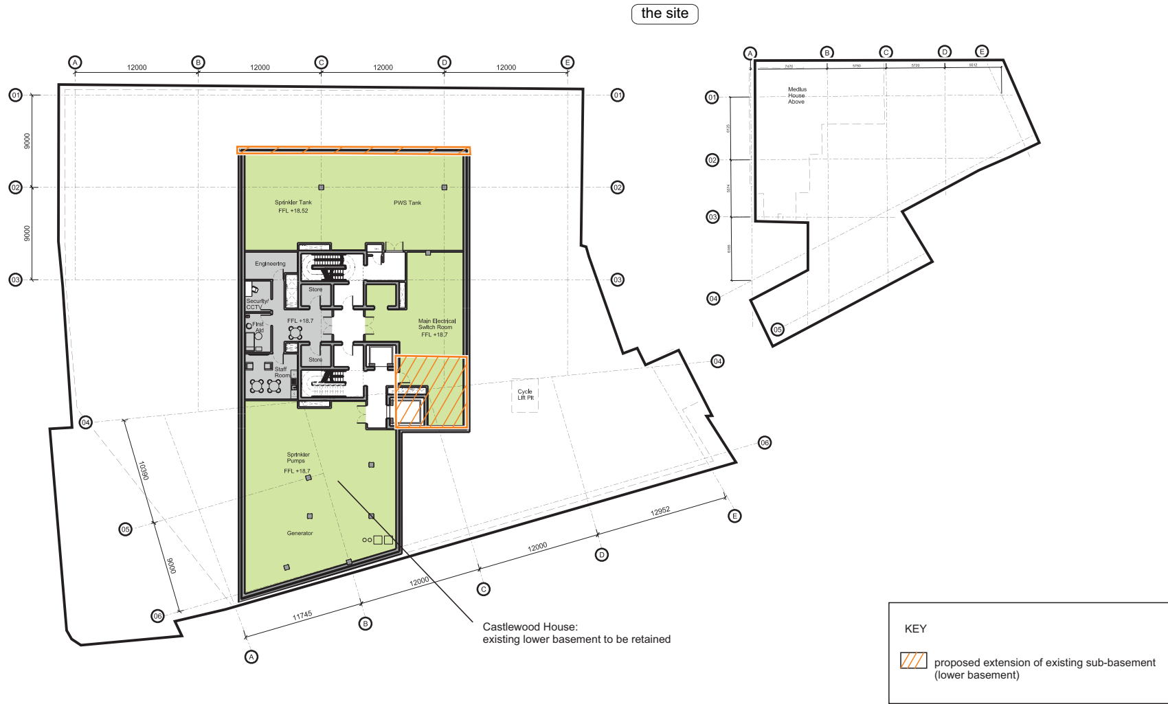
Fig 21 Plan of existing sub-basement to be retained at Castlewood House, showing areas of proposed extension (Robin Partington & Partners, dwg. no. A_PL_P_098, as revised)
