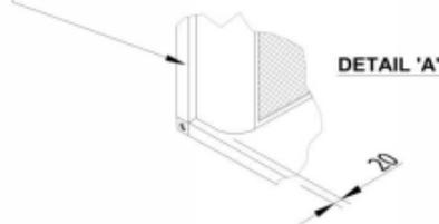
Splitter elements set back in casing by 20mm and provided with aerodynamic bullnoses on inlet and outlet as shown. However if item has non-standard elements refer to Attenuator Model Code Definitions for details.
