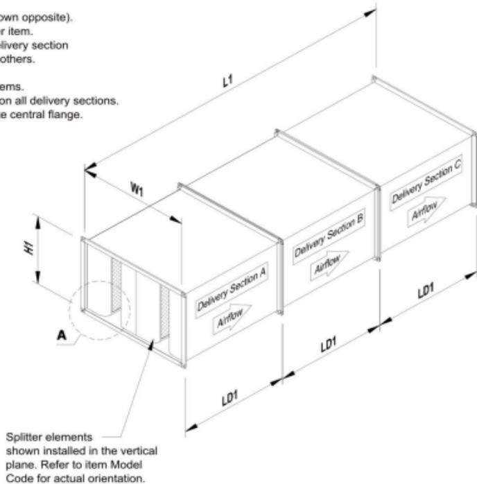
Splitter elements shown installed in the vertical plane. Refer to item Model Code for actual orientation.
