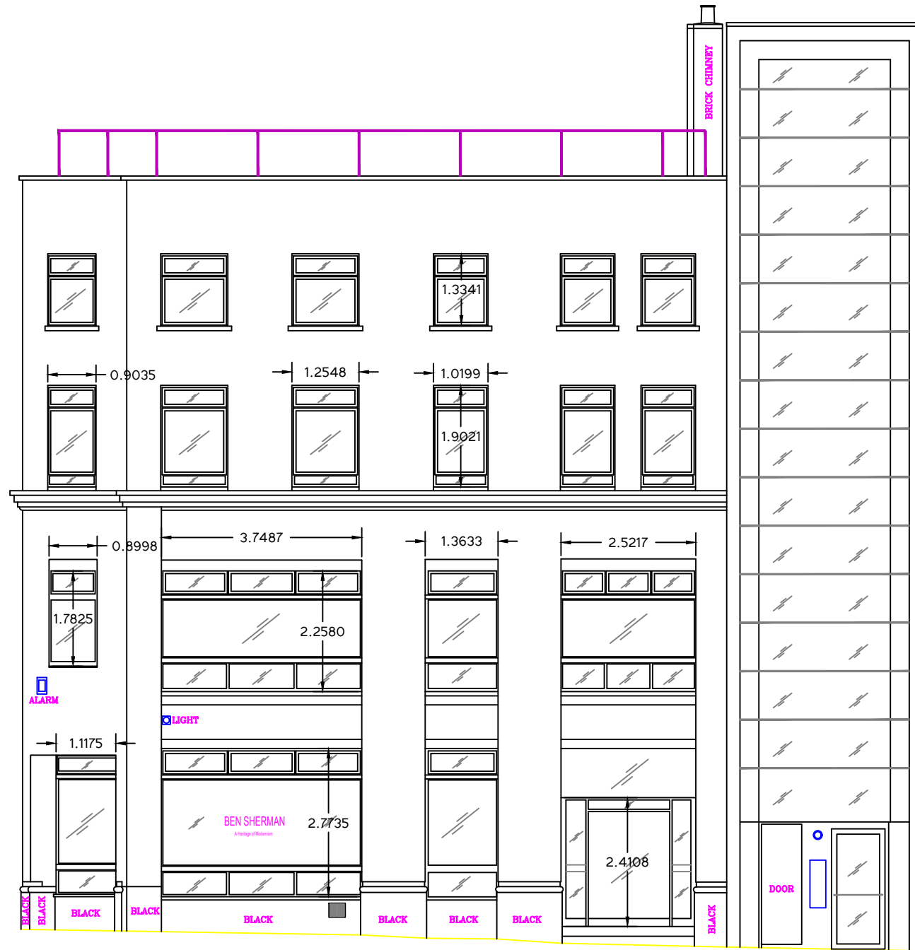
EXISTING ELEVATION TO CLERKENWELL ROAD (C)
