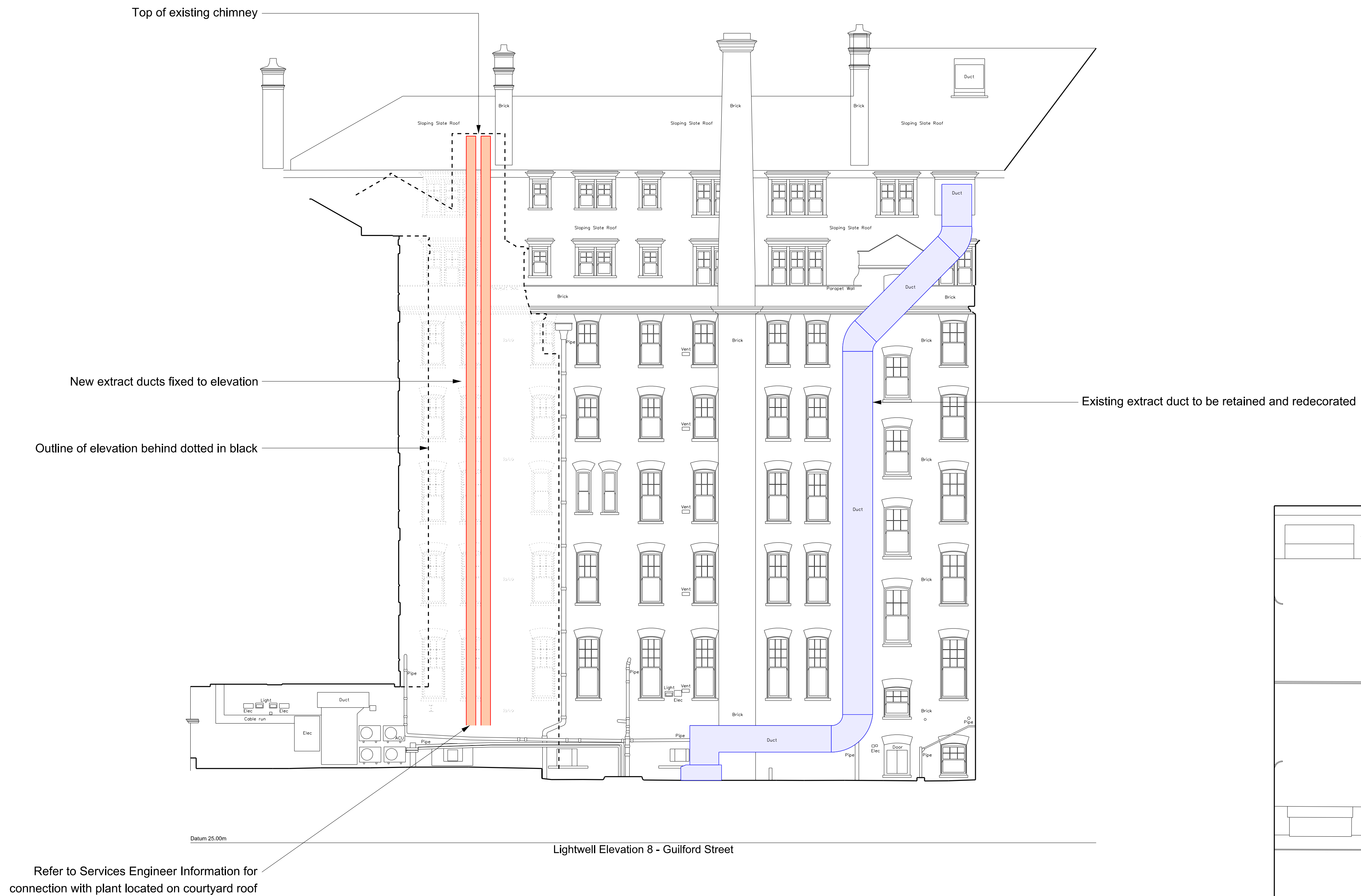
Roof Plan: Extract Ducts in Orange
