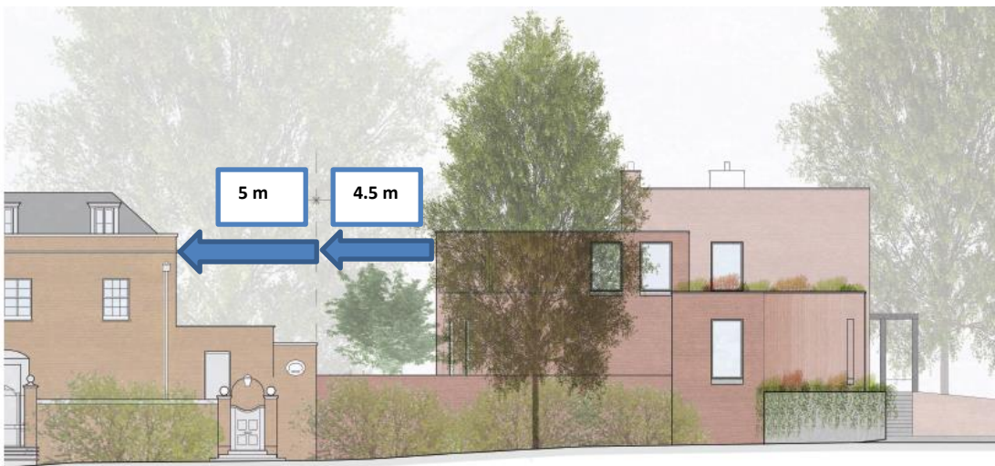
East elevation as proposed with new mass / bulk of rear projection shown
