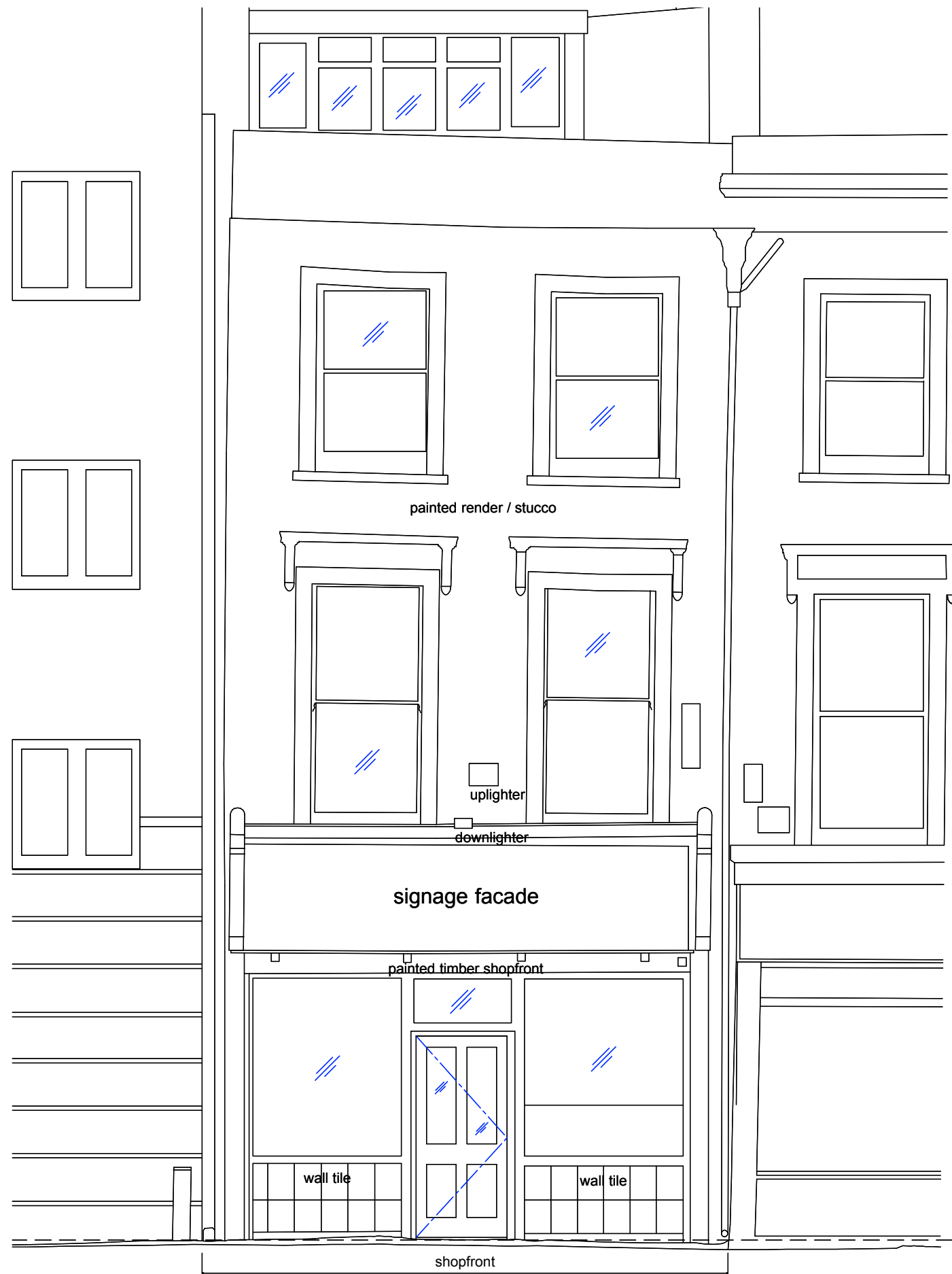
1 Existing Shop Front Elevation 1:50@A3
