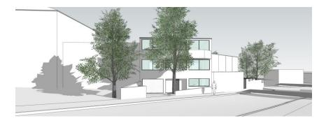
21. The side elevation from the junction shows fixed obscure milky white glass cladding panels set back from the existing brick garden wall.
