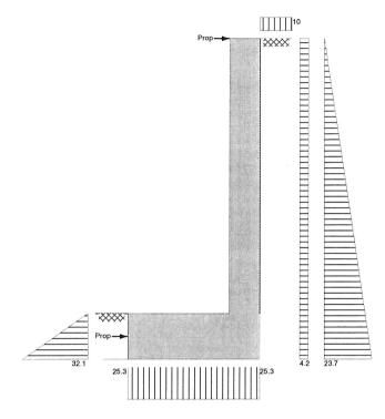
Loads shown in kN/m, pressures shown in kN/m<sup>2</sup>
