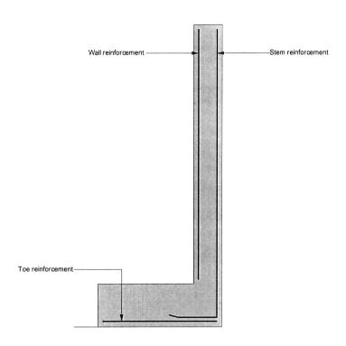
Toe bars - 16 mm dia.@ 200 mm centres -  $(1005 \text{ mm}^2/\text{m})$  Wall bars - 12 mm dia.@ 200 mm centres -  $(565 \text{ mm}^2/\text{m})$  Stem bars - 16 mm dia.@ 200 mm centres -  $(1005 \text{ mm}^2/\text{m})$
