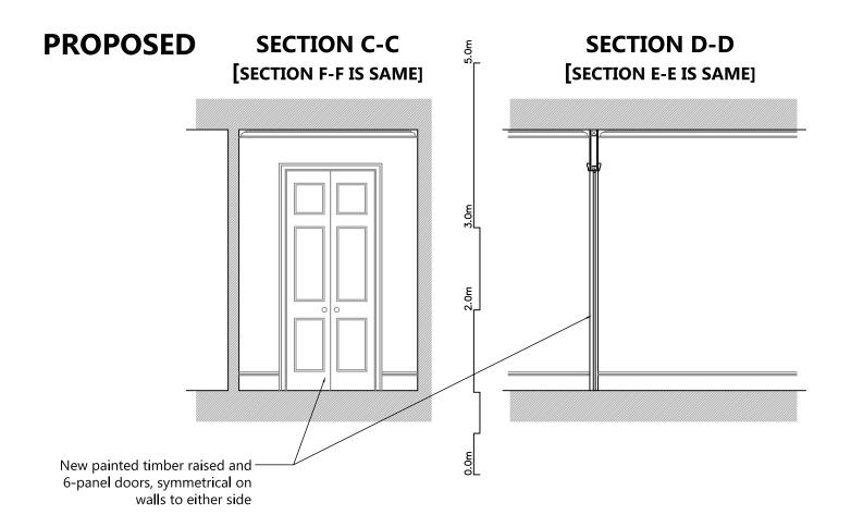
Changes to internal layouts to be undertaken in reversible lighweight stud construction, in timber with surface finishes and decoration to match the existing and original state.
