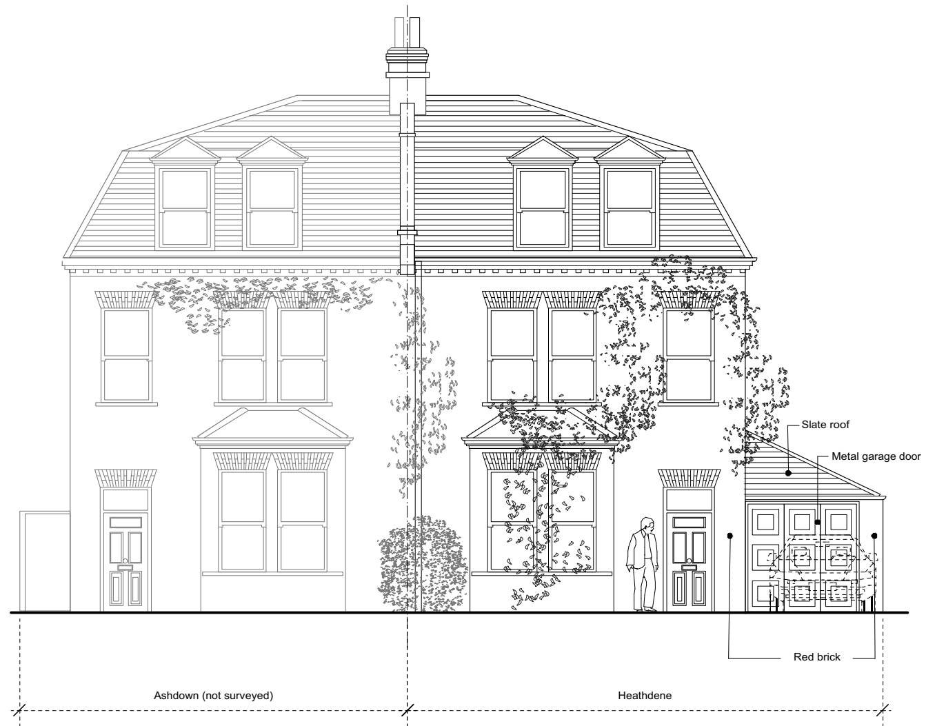
FRONT ELEVATION AS EXISTING 1:100
