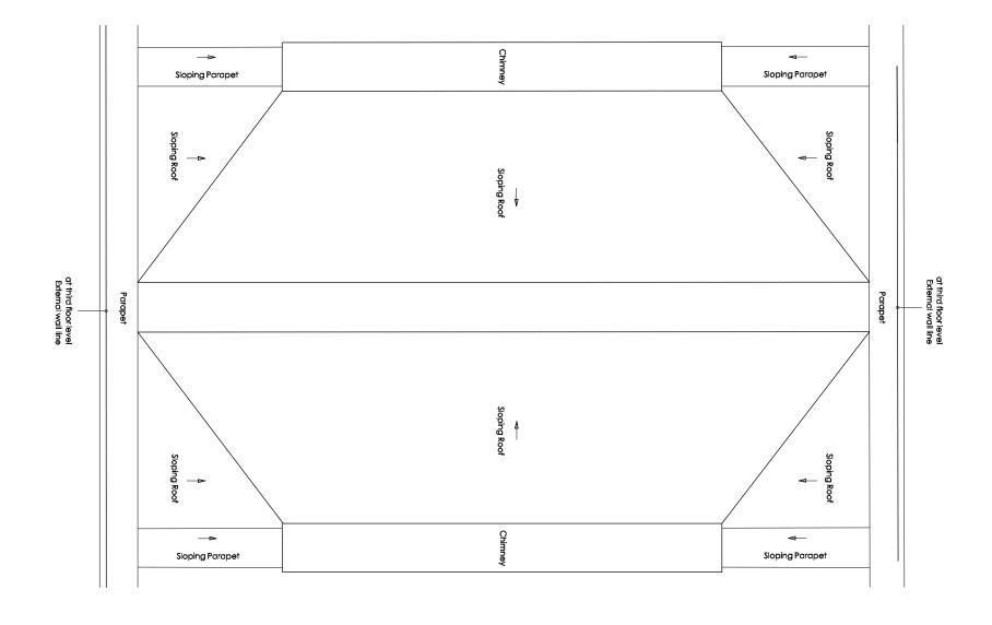
Demolition Roof Plan 1:50
