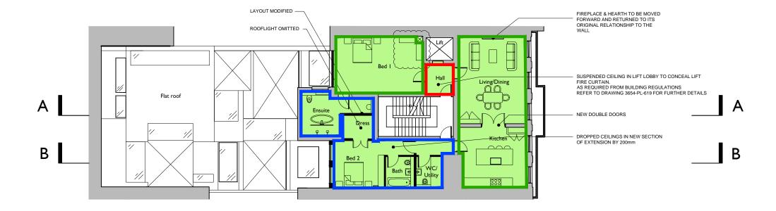
Suspended Ceiling Plan 3654-PL-612 B - SCP FIRST FLOOR PLAN - AS PROPOSED
