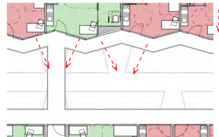
COURTYARD DIAGRAM – CRANKED FACADE HELPS TO MITIGATE OVERLOOKING ACROSS COURTYARD
