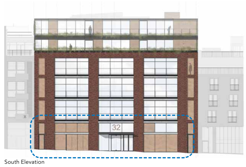
Reynaers Doors: CS77 & CP155LS Hi Elevation and Plan Details
