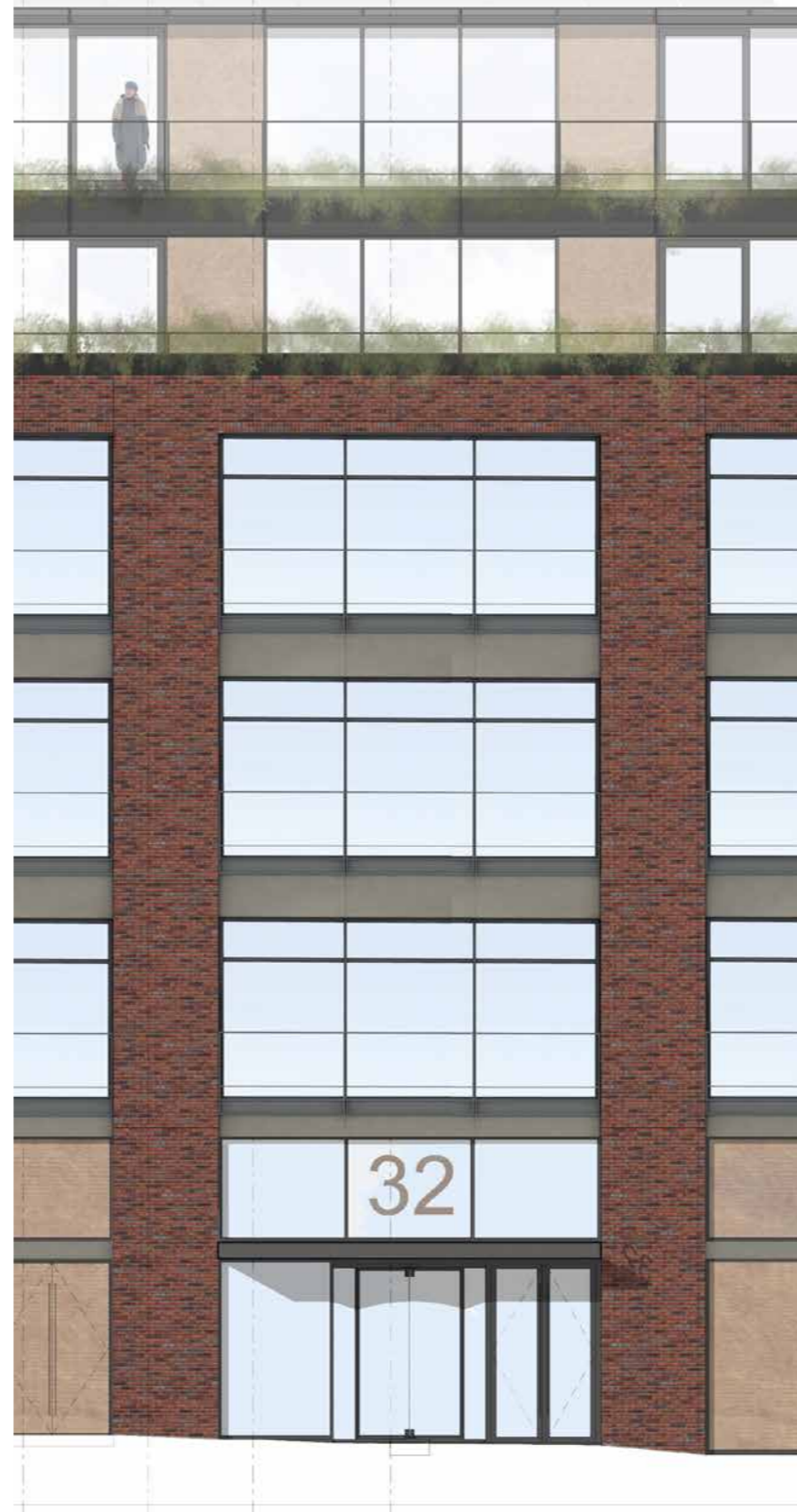
South Elevation - Proposed Curtain Walling
