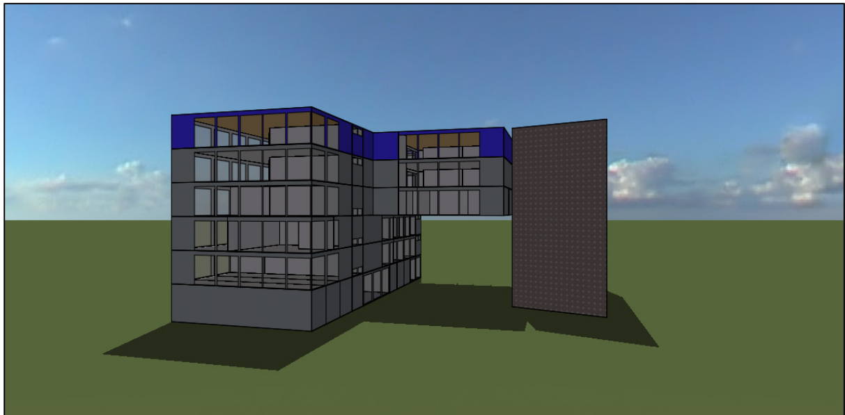
Figure 1: New Level (shown blue), Roundhouse Administration Building – 3D Engineering Model
